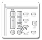
▶ Press the **Air Swing** (≥ button one more time to set the air flow direction, when the blade reaches the desired position. The up/down tilting of the blade will stop in place.
